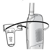
**To remove the belt clip**Pull the left edge in the direction of the arrow.
